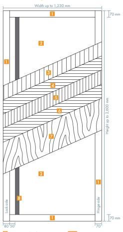
1 Framing/timber2 Sandwich system with high heat insulation
